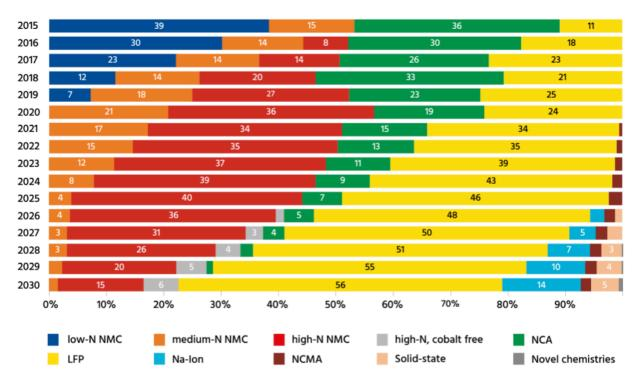
Figure 4. Forecast of battery chemistry usage. Source: Rystad Energy.
